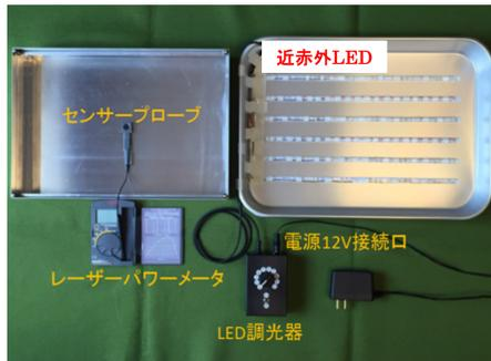
Near-infrared ray irradiation device
