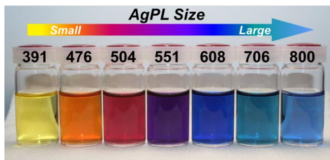
Fig. 1: The aqueous dispersion for different-sized AgPL. The peak wavelengths of LSPR in their UV/Vis/NIR extinction spectra are shown in nanometer.
